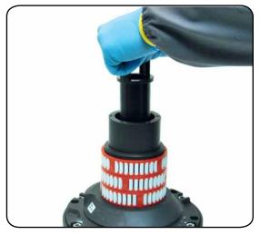
7. Slide out the assy clutch  $n^{\circ}36$
