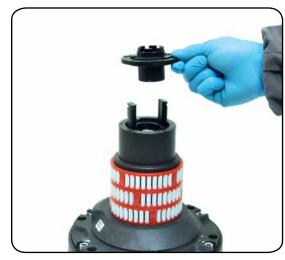
6. Remove the stripper arm housing n°21
