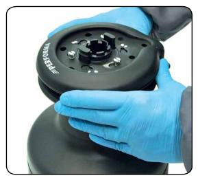
When positioning the stripper arm, align the peeler with it. If the jaws have been disassembled, insert peeler between the two jaws, taking care that the letters TOP on the peeler
