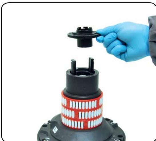
6. Remove the stripper arm housing n°21
