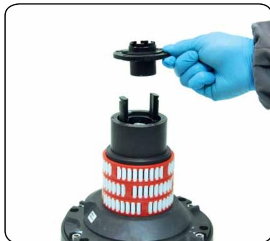
6. Remove the stripper arm housing n°21
