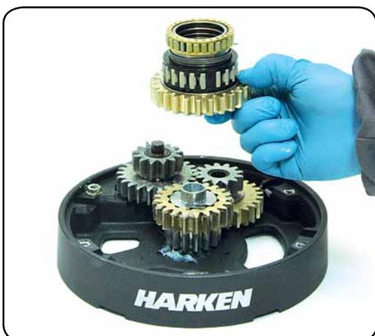
11. Remove the gear n°30, pawls carrier n°32, the bearings n°33 and 35 and the pin n°34. Important: washer n°7 may remain inside the drum support!
