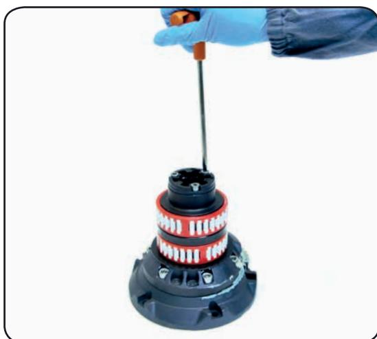
4. Completely unscrew the three screws n° 26 and remove the socket support
