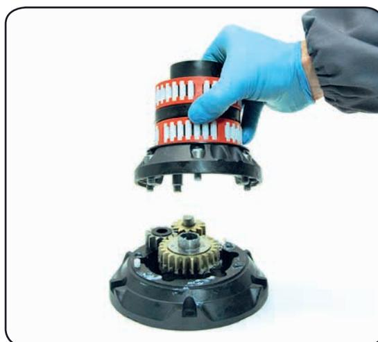
7. Remove the assembly housing n° 16.
