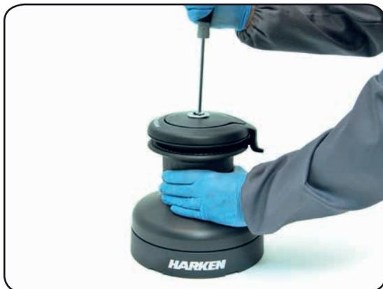
1. Unscrew the central screw ( $\approx 2\text{Nm}/18\text{ in-lb}$ )
