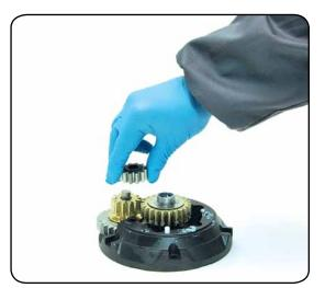
10. Remove the gear  $n^\circ 15$
