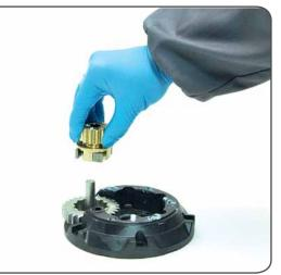
14. Remove the pinion  $n^{\circ}10$ .
