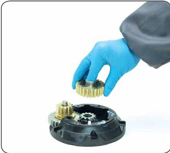
12. Remove the gearing n°9 and remove the pawls n°7. To facilitate the operation press the spring against the pawl with a blade.
