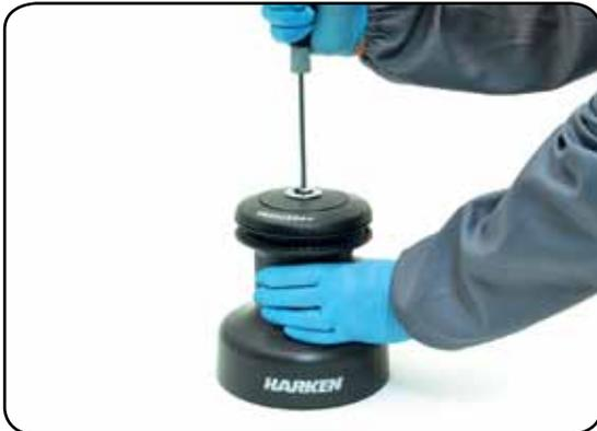
1. Unscrew the central screw ( $\approx 2\text{Nm}/18\text{ in-lb}$ )
