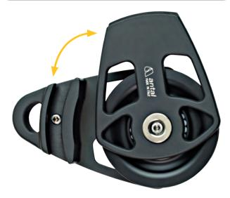
The cheekplate revolves around the sheave axle allowing the block to open; a safety pin, which engages automatically on closing, stops the block from opening accidentally.
