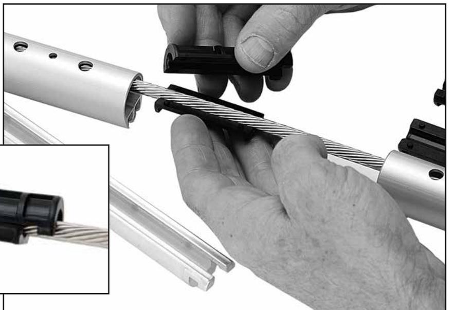
Slip 9" (229 mm) connector on wire, mating hook of plastic bushing with connector.
