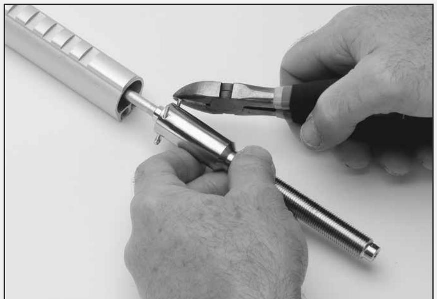
Assemble turnbuckle and attach Harken toggle.
