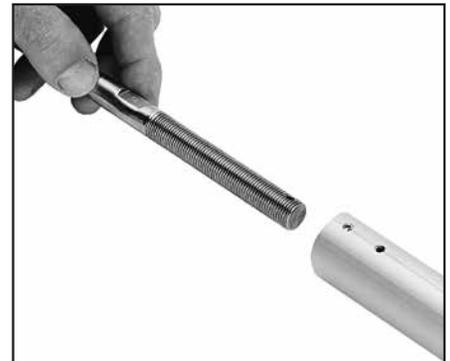
**! WARNING! Using a threaded nosepiece with only adhesive at the upper rod eye terminal may result in headstay system failure. Make sure there is a mechanical lock.**
