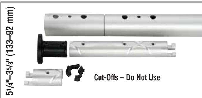
5<sup>1</sup>/<sub>4</sub>"–3<sup>5</sup>/<sub>8</sub>" (133–92 mm) Do not use plastic bushing above top connector. Cut connector right at cross formed by glue dispersion channels. Use single foil screw in top foil only.
