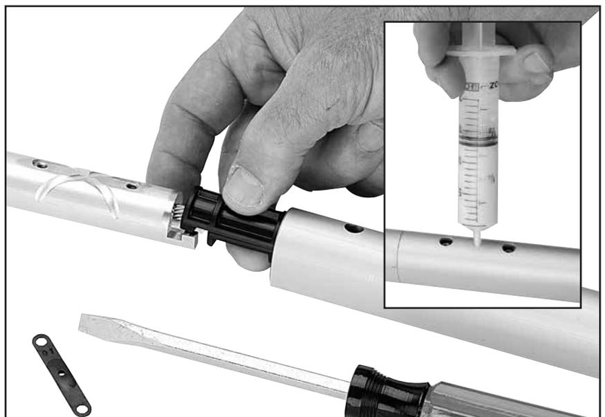
Continue installing connectors and wedges. Make sure to use red Loctite® in screw holes.
