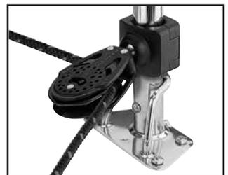
**Lead line through block so ratchet makes clicking sound when pulling line to furl sail.**
