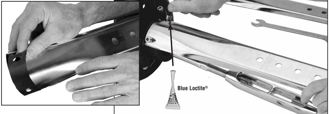
Fasten second long link plate to drum assembly and secure to clevis pin using locknuts.
