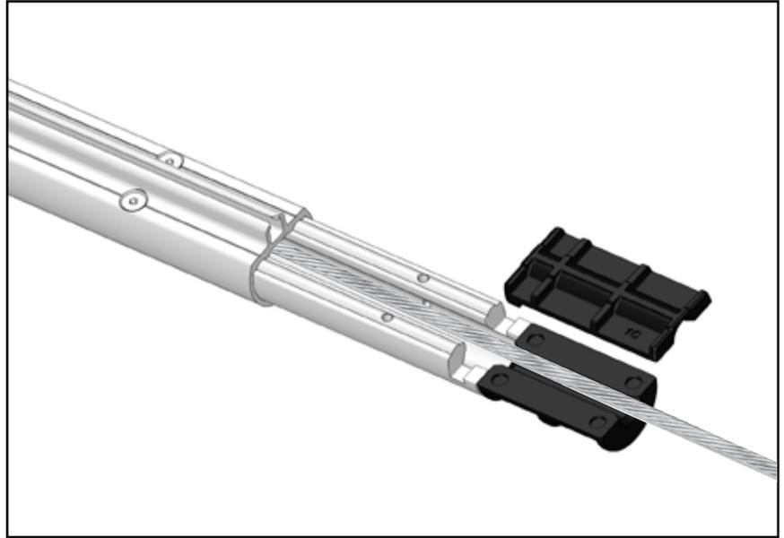
Put a drop of red Loctite® into screw holes.
