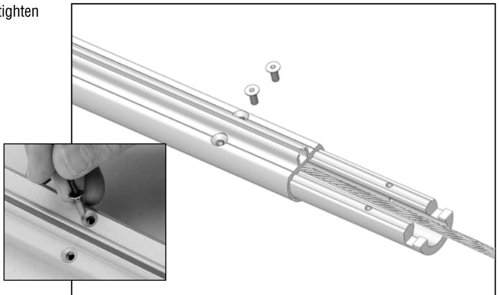
Sandwich bushings on wire, mating hook of plastic bushing with connector and mating with four recesses in bottom part of bushing.
