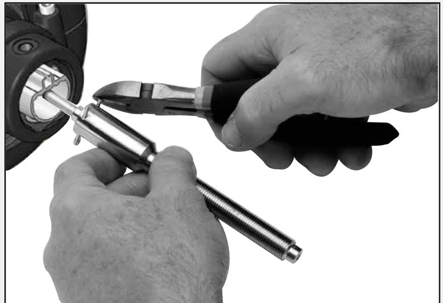
Assemble turnbuckle and attach Harken toggle.
