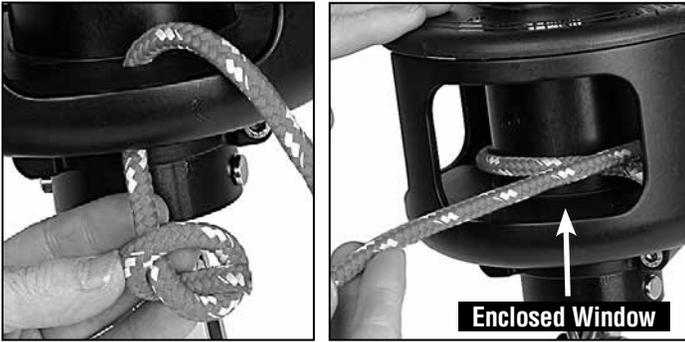
Run line through enclosed window in guard and into hole in bottom plate of spool. Tie a small overhand knot and pull it up under drum assembly.
