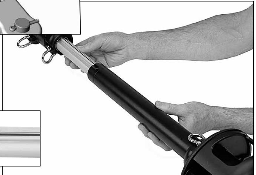
Secure using hex key. Use Tefgel on screws. **NOTE:** You will likely adjust foil height again once system is up on the mast and turnbuckle adjusted.
