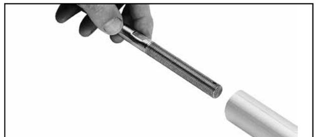
**WARNING!** Using a threaded nosepiece with only adhesive at the upper rod eye terminal may result in headstay system failure which can cause an accident, damage to your vessel, personal injury, or death. See [www.harken.com/en/general-warnings-instructions/](http://www.harken.com/en/general-warnings-instructions/) for additional safety information.
