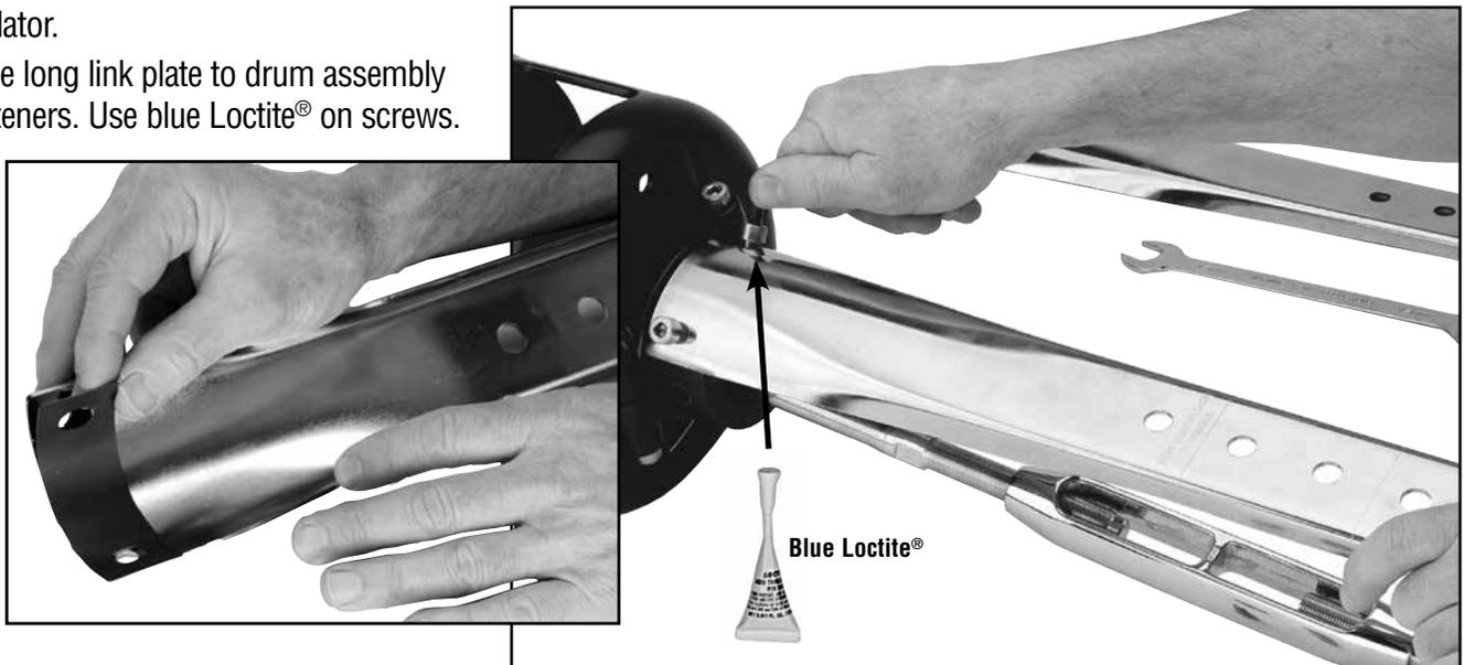
Fasten second long link plate to drum assembly and secure to toggle using locknuts.
