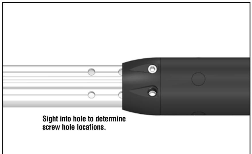
Slide halyard swivel above feeder. Place feeder tabs in position. Use a drop of 833 Blue Loctite® in screw holes. Use hex key wrench to secure.
