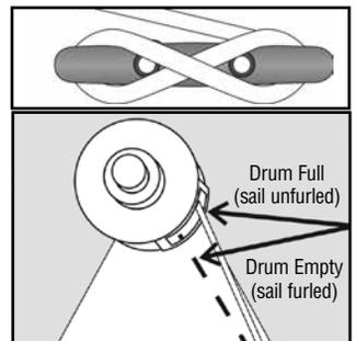
**Note:** As furling line lead changes, make sure line doesn't chafe against line guard. Rotate line guard if necessary.
