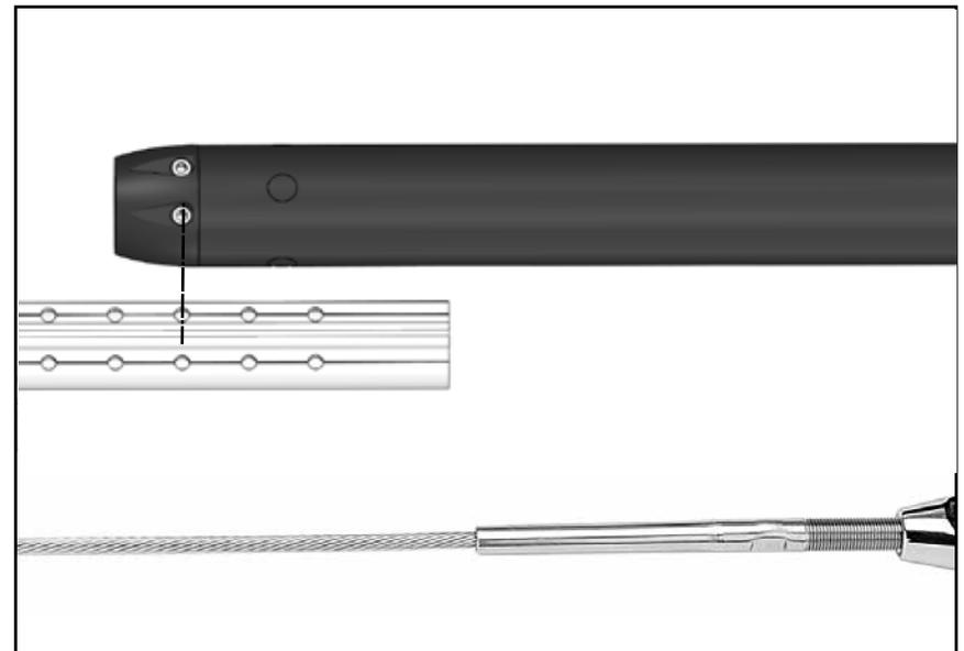
**Note:** Position top foil so that with top cap the foil will ride 5/8" (16 mm) below terminal. If wire fitting at top of stay is swage, foil must ride just below shoulder of swage. Mark cut line on foil. Wrap tape around foil as a guide so cut is straight.
