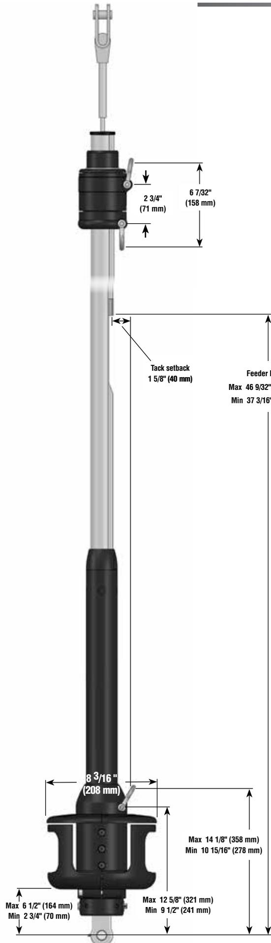
**Long link plate note:** If a long link plate is used, add the following dimensions to feeder, tack shackle, and drum height (based on whether plate is used full-length or shortened to one of five hole positions). Do not add to halyard swivel or top terminal dimensions.
