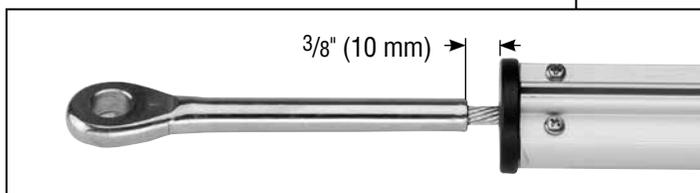
Secure using hex key. Use Tef-Gel on screws. **NOTE:** You will likely adjust foil height again once system is up on the mast and turnbuckle adjusted.
