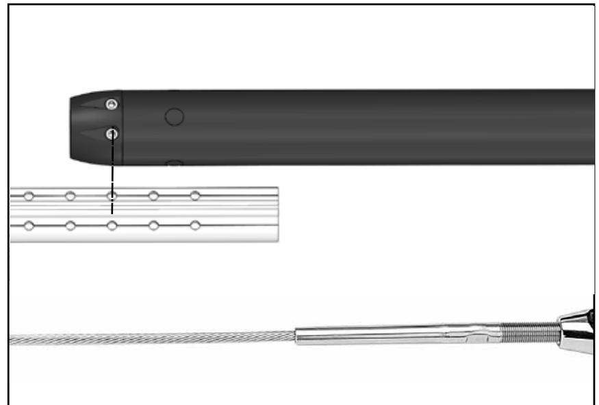
**Note:** Position top foil so that with top cap the foil will ride 3/8" (10 mm) below terminal. If wire fitting at top of stay is swage, foil must ride just below shoulder of swage. Mark cut line on foil. Wrap tape around foil as a guide so cut is straight.
