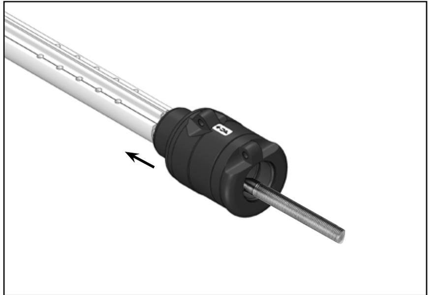
Slide drum assembly onto foil.
