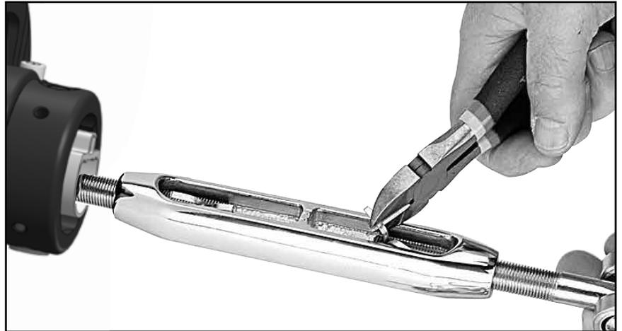
Slide lower drum assembly over turnbuckle and attach using long crosspin. Use plastic washers provided.
