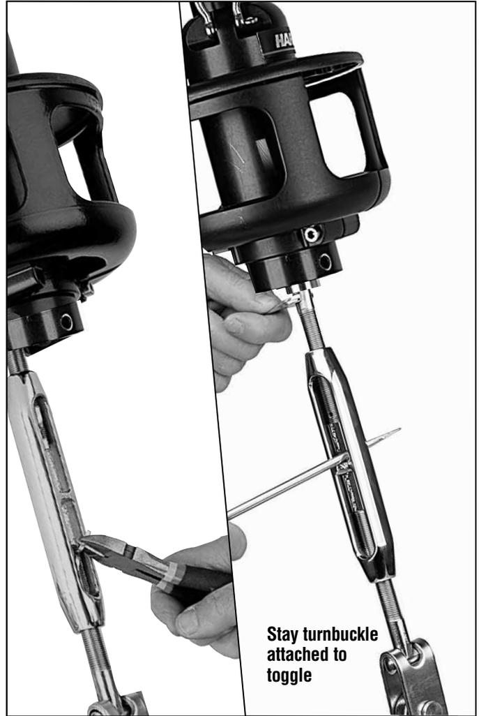
Lift foils so top is  $\frac{3}{8}$ " (10 mm) below upper terminal. Use Tef-Gel on foil clamp screws when you replace them.
