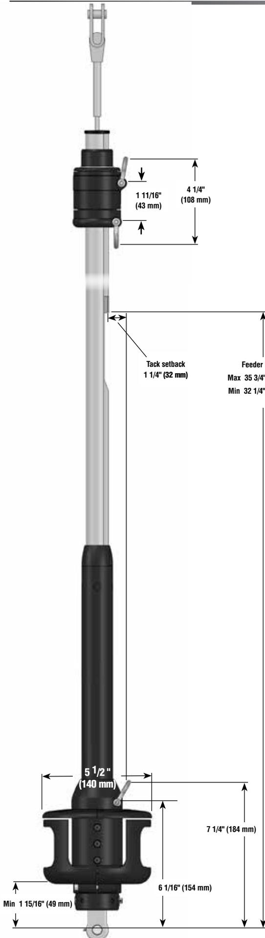
Use dimensions of Harken toggle below to build stay to correct length.
