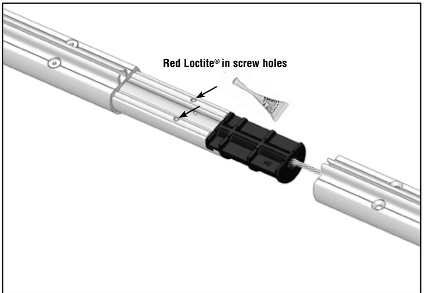
Slide foil completely over bushings and connector. Use a hex key wrench to securely tighten screws. **Continue assembly of foil system.**
