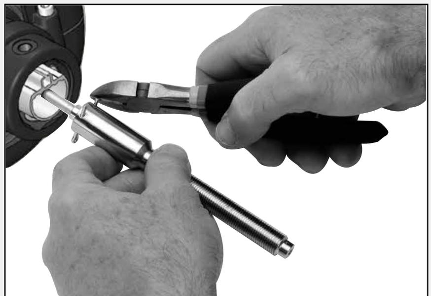
Assemble turnbuckle and attach Harken toggle.
