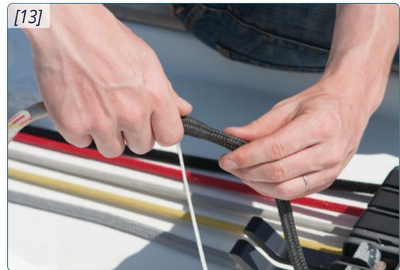
14 Hook the elastic loop to the end of the textile sleeve. This pre-tension on the sleeve helps to ensure a positive initial grip when transferring the load on the line or halyard from the winch to the Constrictor®. Manually "milking" the textile sleeve in the direction of the load prior to releasing from the winch will minimise movement of the line as the load is taken up by the Constrictor®.
