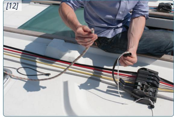
13 Thread the rope through the entire length of the textile sleeve until it comes out the other end of the body.
