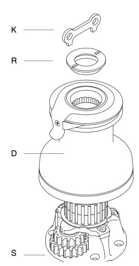
1 The installation of the XT winch requires that you lift the drum. First of all, unscrew the upper ring (R) with the provided key (K). Thus lift the drum (D) to access the anchoring holes on the skirt (S) of the winch.
