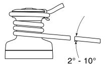
Placement of the skirt. Position the winch so that the output gear is in the area shown in the figure, i.e., tangent to the pull direction of the maneuver.
