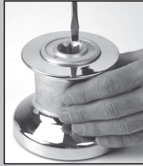
Use screwdriver to open winch.
